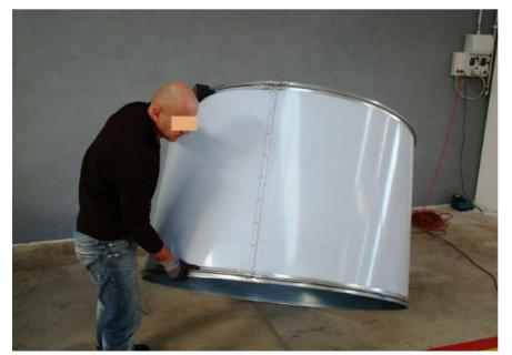
In an average time of 2-3 minutes of assembly, the duct is now ready to be mounted.
